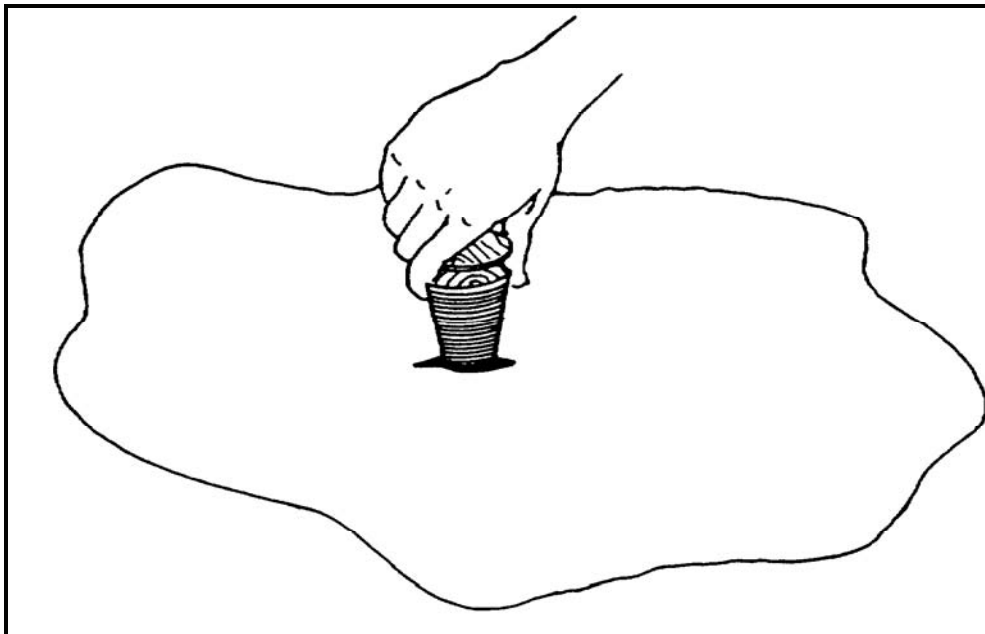
Figure 1. Wood plug repair.
